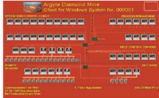
Graphic display of the mine's automated treatment process
