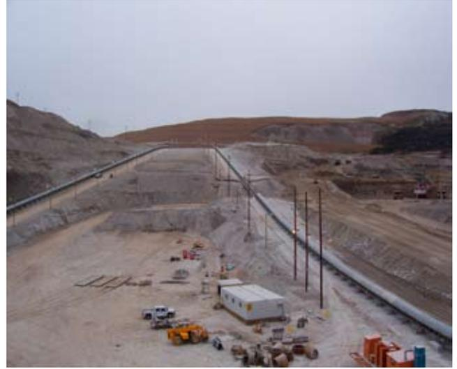
Conveyors move 6000 tons of coarse ore per hour
